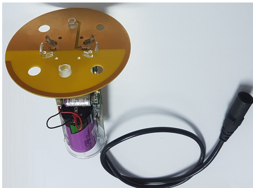
Antenna- Top Assembly
