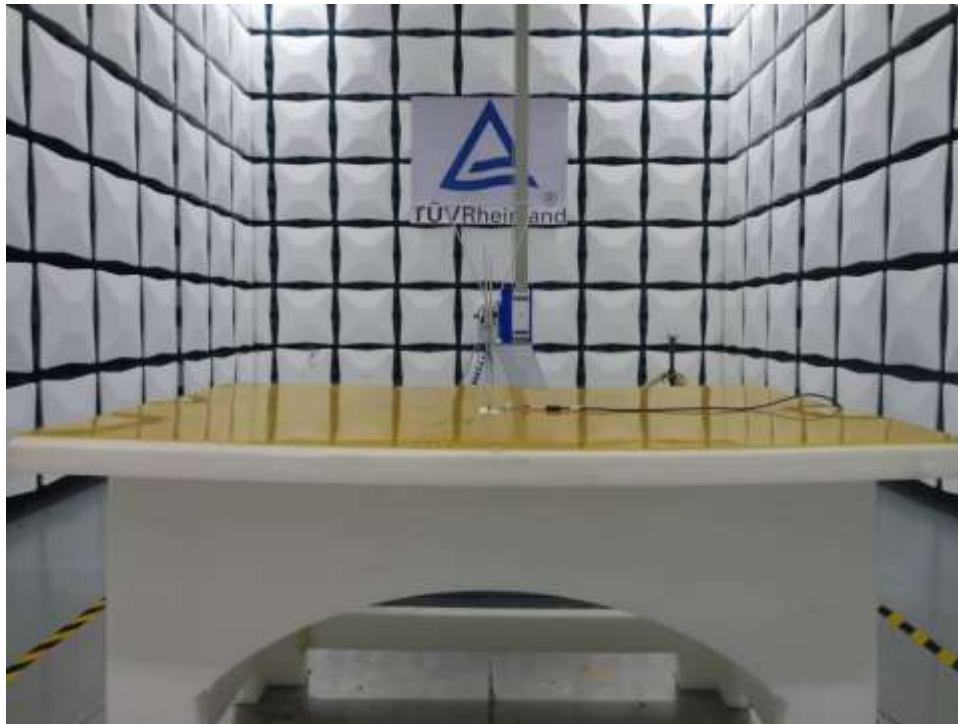
Photograph 1: Set-up photo for Radiated Emissions Below 1GHz
