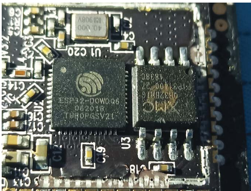
EUT – IC Chip View (for Main Board 1)
