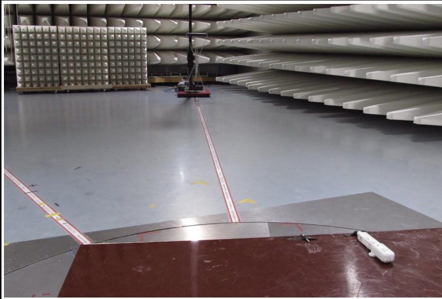
Test setup configuration 4 antenna VULB 9126 vertical AC 6
