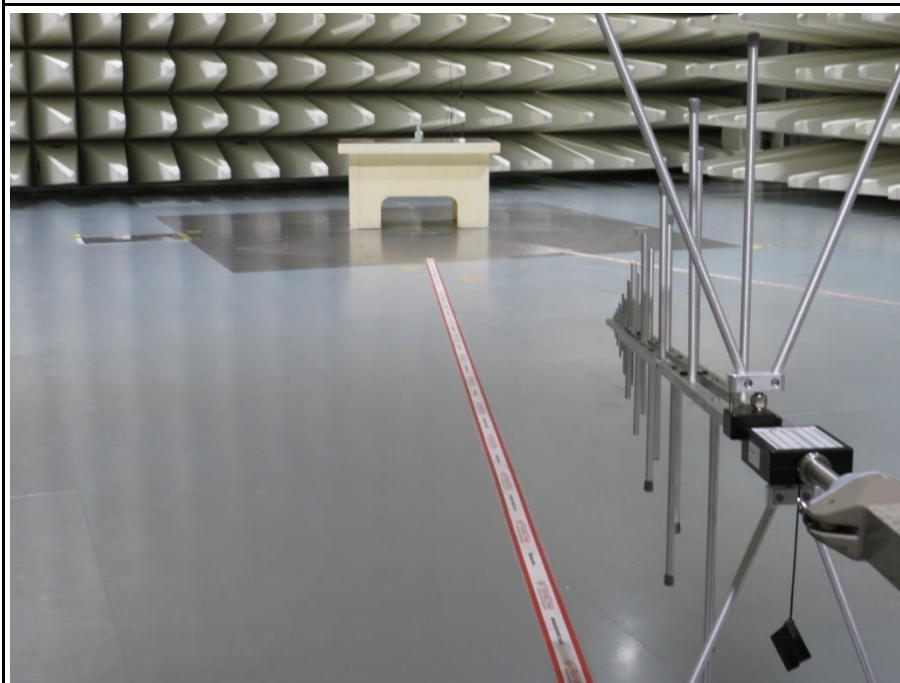
Test setup configuration 2 antenna VULB vertical AC 6
