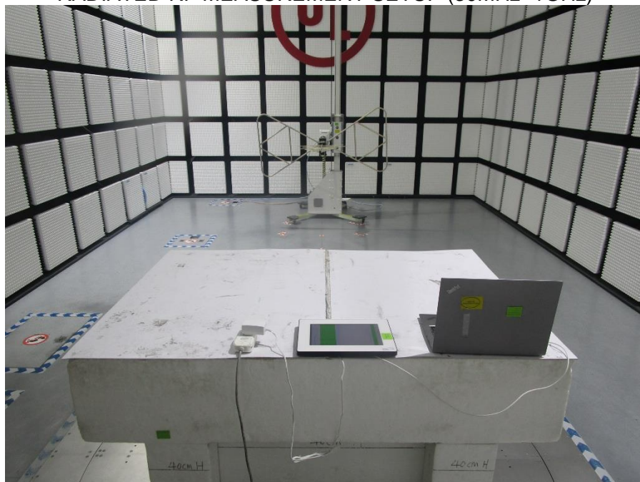
RADIATED RF MEASUREMENT SETUP (Below 30MHz)
