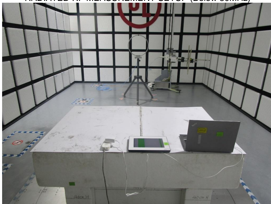
RADIATED RF MEASUREMENT SETUP (Below 30MHz)
