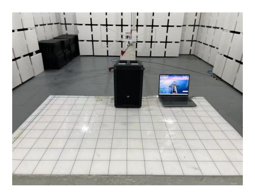
Set-up for Radiated Spurious Emission, Above 1GHz
