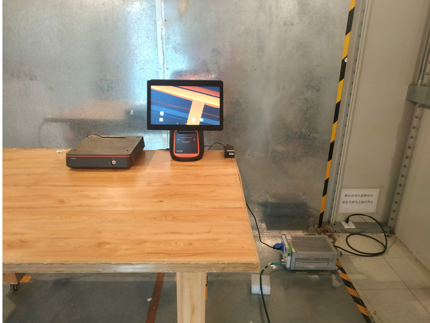
Conducted Emissions (Side View)
