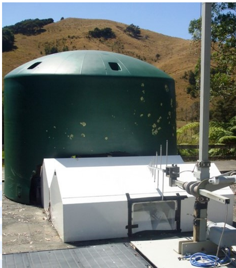
Test shed showing the use of a log periodic antenna
