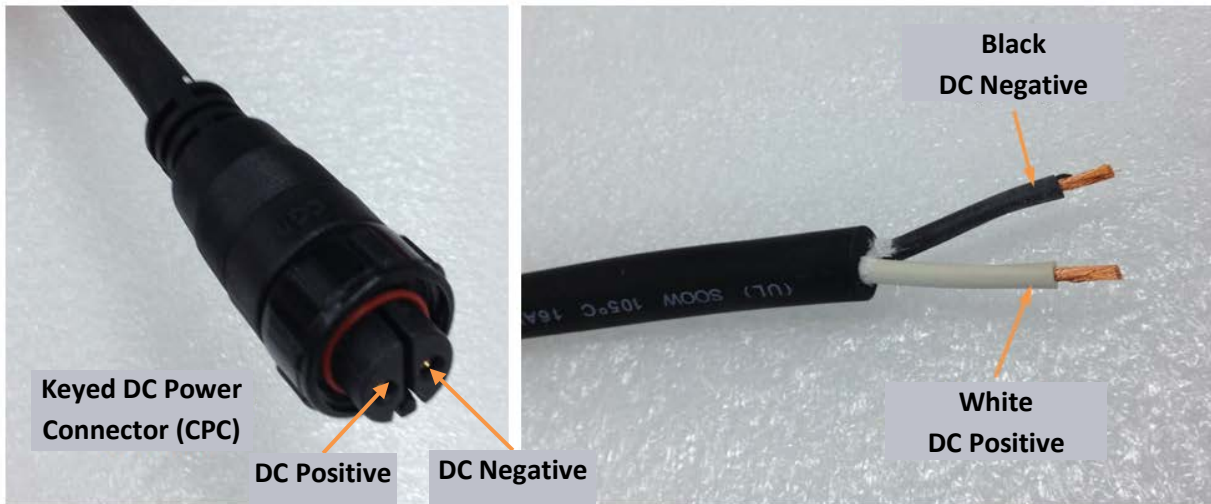
Figure 14: Mobile Gateway Module DC Power Connector Signals
