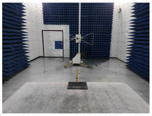
RADIATED EMISSION TEST SETUP ABOVE 1GHz
