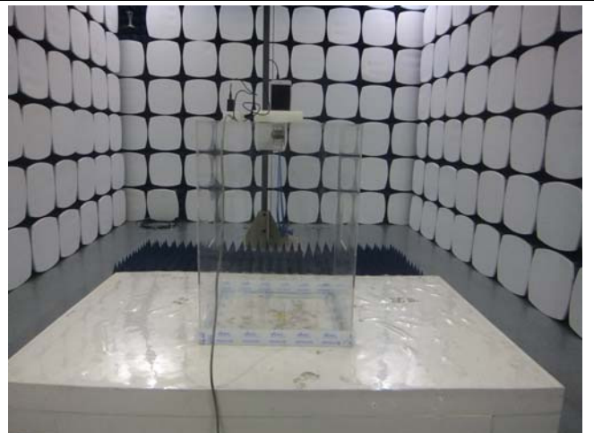
Radiated Spurious Emissions Test Setup Above 1GHz
