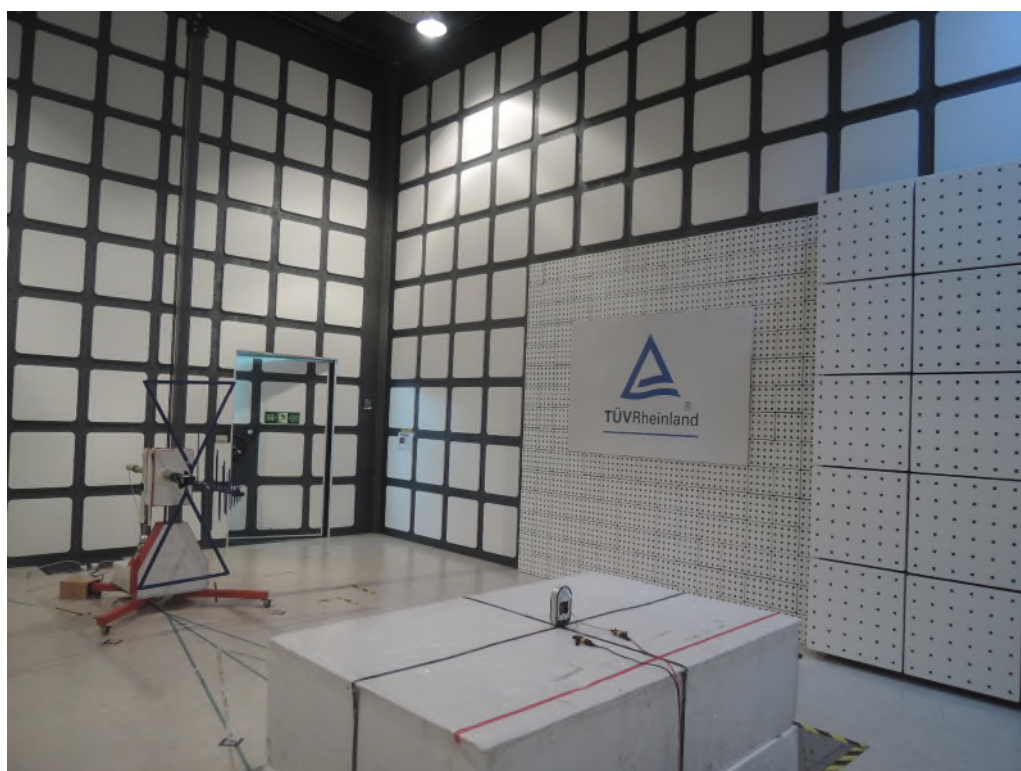
Photograph 2: Set-up for Radiated Emissions (Back View 1)
