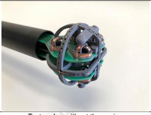
Test probe, without the casing
