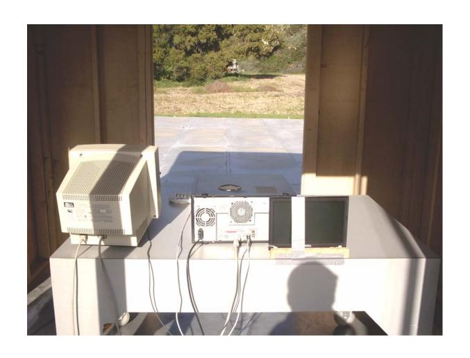
Radiated Emissions Measurement (Rear View)
