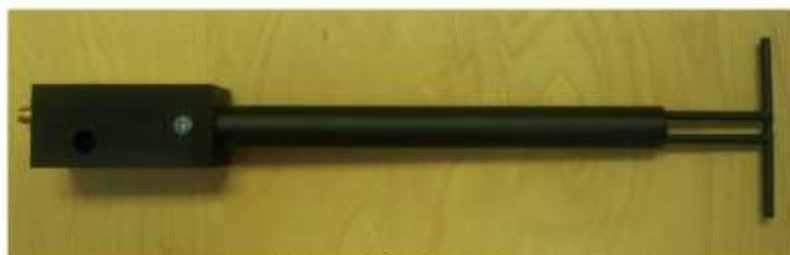
Figure 1 – MVG COMOSAR Validation Dipole
