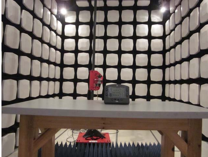
Measurement of Radiated Emission Test Set Up
