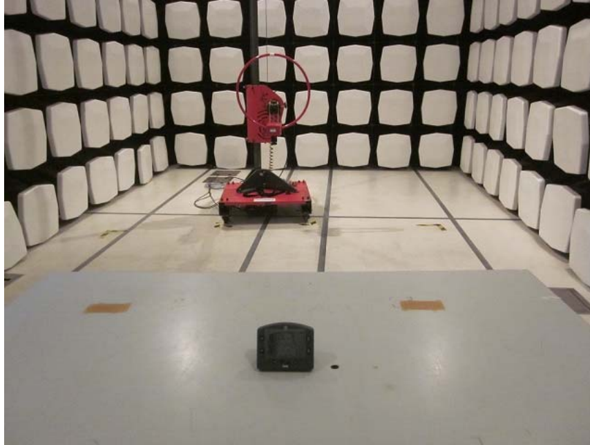
Measurement of Radiated Emission Test Set Up
