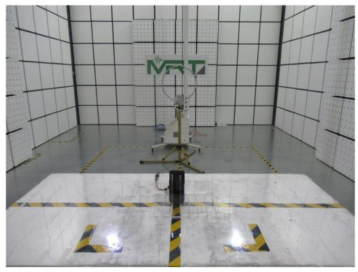
Description: Radiated Spurious Emission Test Setup for 30MHz ~ 1GHz
