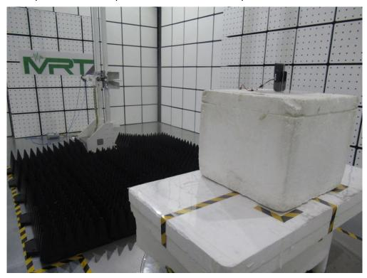
Description: Radiated Spurious Emission Test Setup for  $18\text{GHz} \sim 25\text{GHz}$
