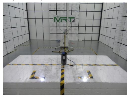
Mode 2 Description: Radiated Spurious Emission Test Setup for 30MHz  $\sim$  1GHz
