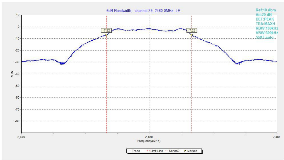
Fig.22. 6dB Bandwidth: GFSK, 2480 MHz
