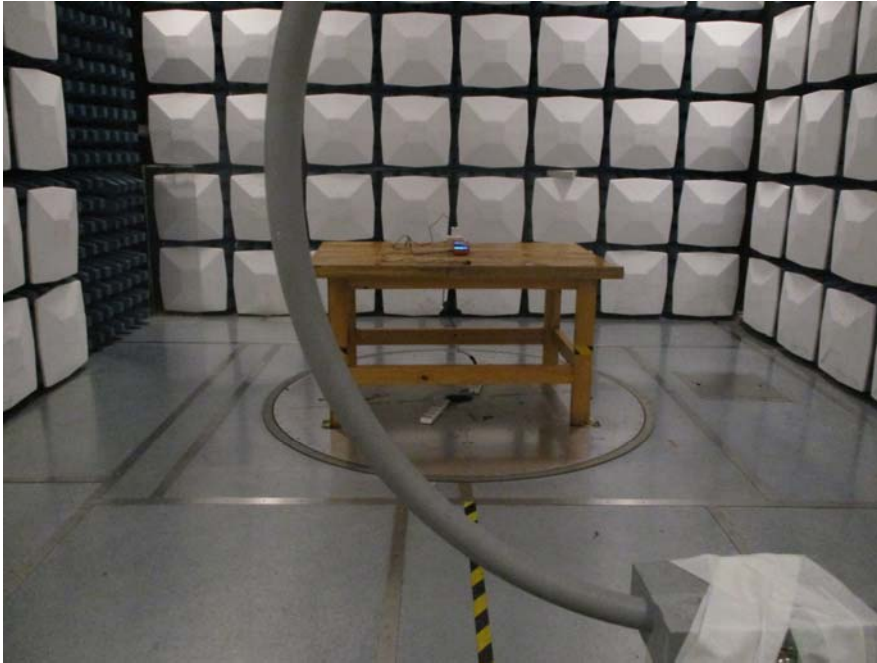
Radiated Emission-View (9 kHz~30 MHz)
