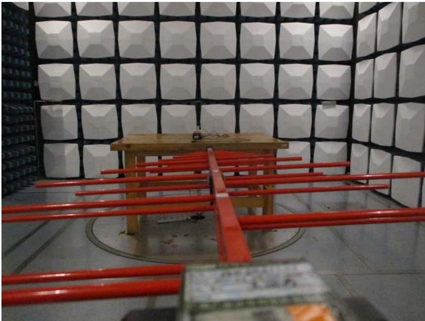
Radiated Emission- View (30 MHz ~1 GHz)
