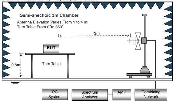
(C) Radiated Emission Test-Up Frequency Above 1GHz
