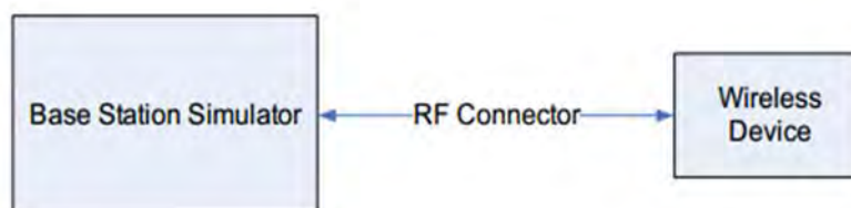
Figure 9.2 Power Measurement Setup
