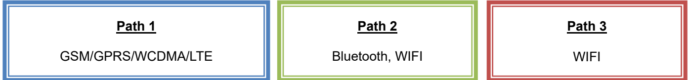
Figure 12.1 Simultaneous Transmission Paths
