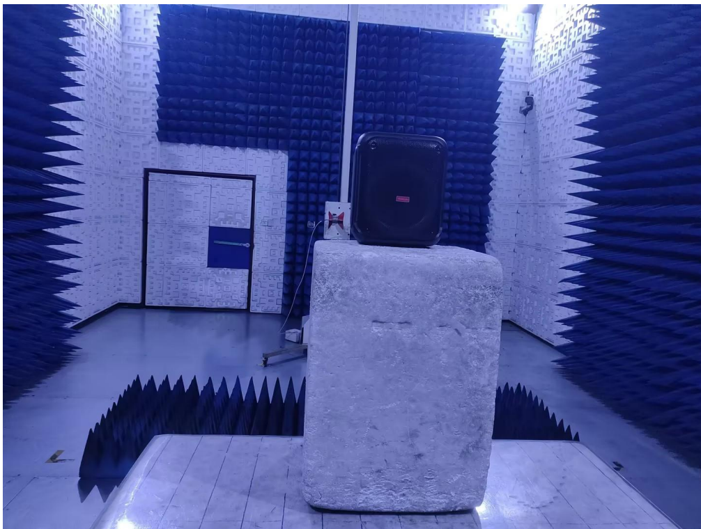
RADIATED EMISSION TEST SETUP ABOVE 1GHz
