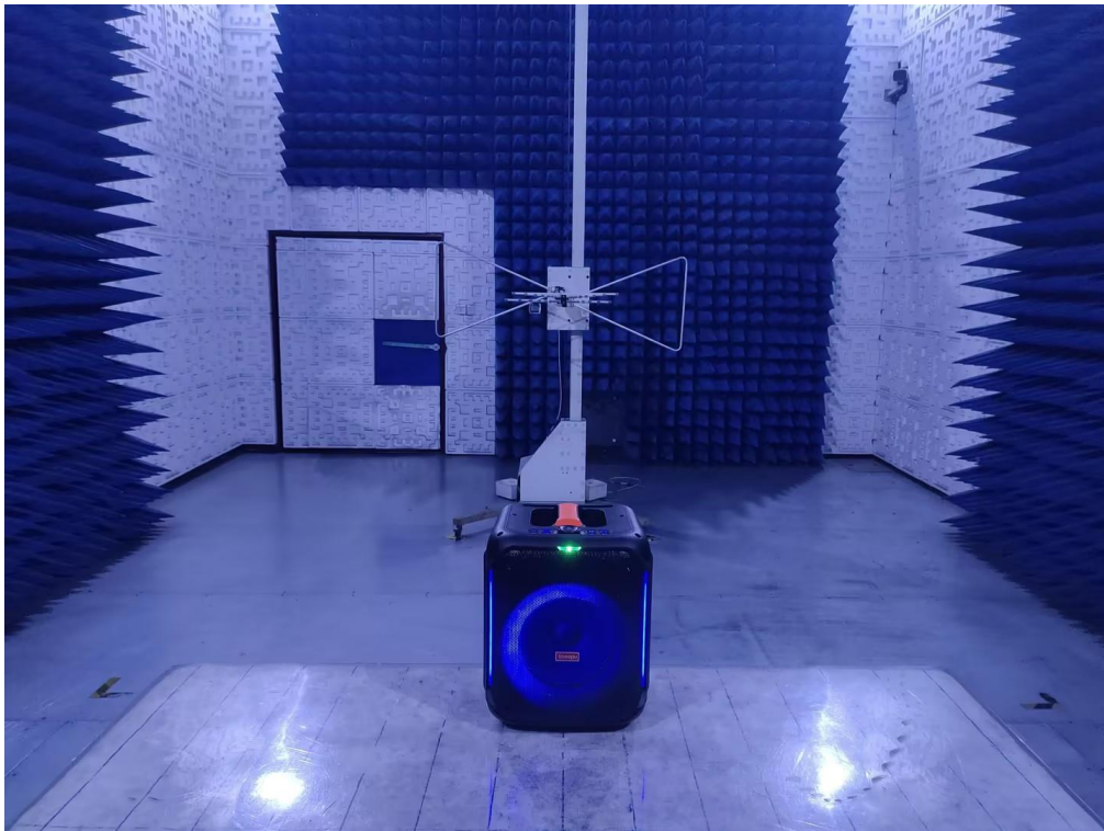
RADIATED EMISSION TEST SETUP ABOVE 1GHz
