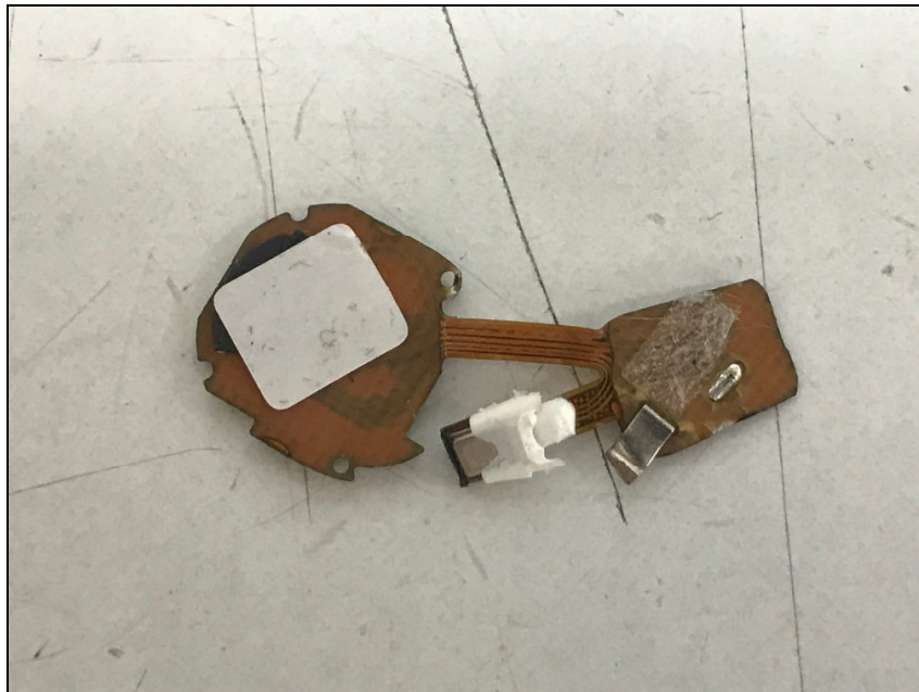
Bottom view of Sub PCB
