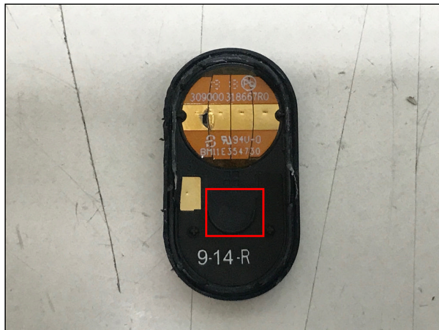
View of Bluetooth antenna
