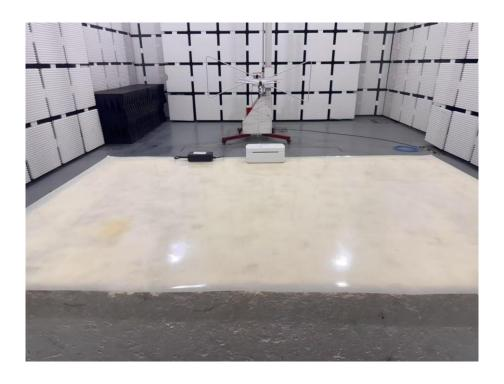
**Set-up for Radiated Spurious Emission, Above 1GHz**
