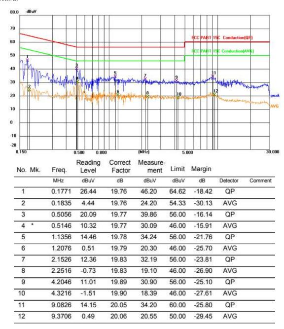
\*\*\*Note: 1).Pre-scan all modes and recorded the worst case results in this report BT LE-1M (Middle Channel). 2). Result = Reading + Correct, Margin = Result - Limit.
