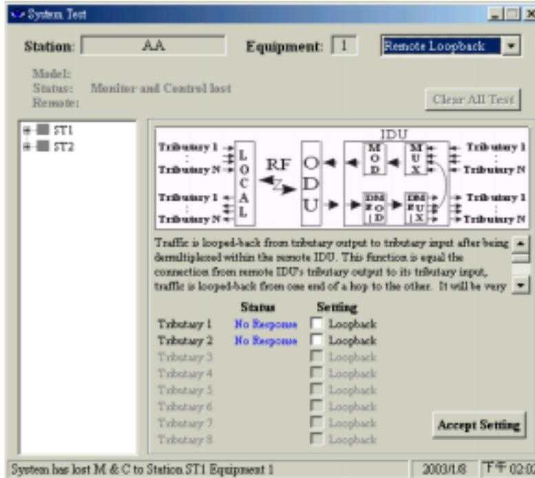
While performing remote loopback function test, first select the testing tributary. Press Accept Setting to execute this function. Press Close All Test to end the test.
