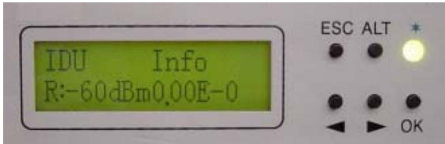
1. First line of the LCD display - On the right hand side, in every alternate 1~2 seconds, it displays the I-Temp: xx.x□ stands for IDU temperature. O-Temp: xx.x□ stands for ODU temperature. On the left hand side, 4E1 stands for the activity measure.
