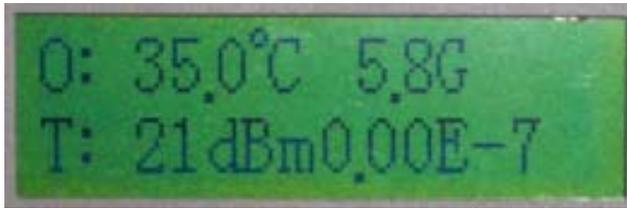
Under normal working condition, display the indoor and outdoor temperature, receiving power and online BER. The display refresh every 1~2secs.
