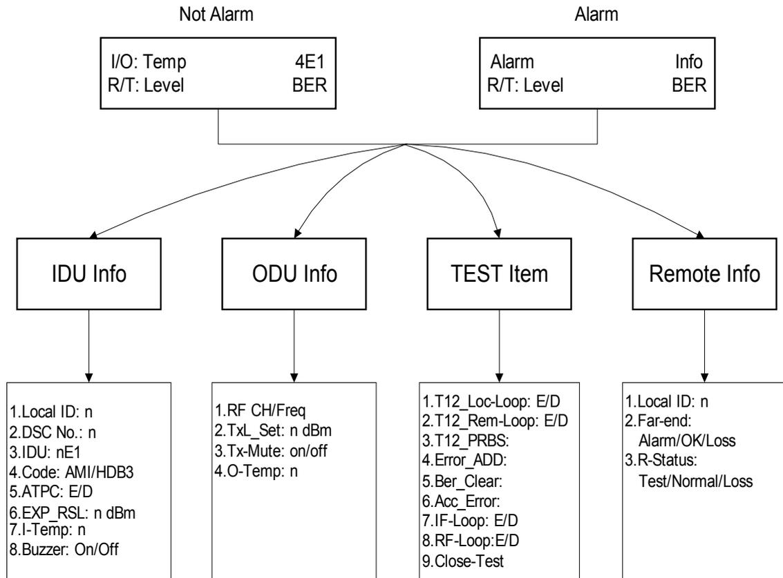
**Under normal condition (no alarm), the LCD displays as below:**
