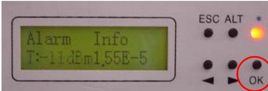
Now press the OK button of the panel. It will display the alarm message. Press the Right/Left button of the panel. The LCD displays the present alarm/warning message.
