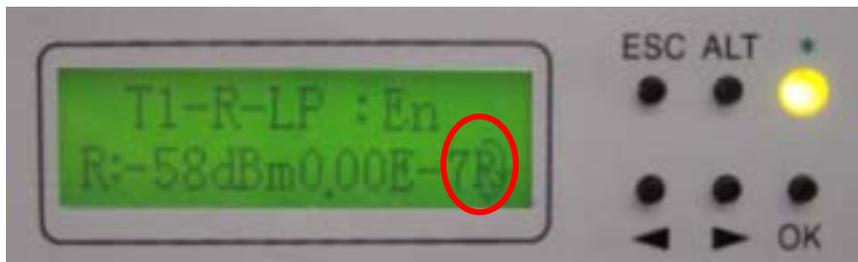
Remote end: The right bottom side displays a loopback sign.
