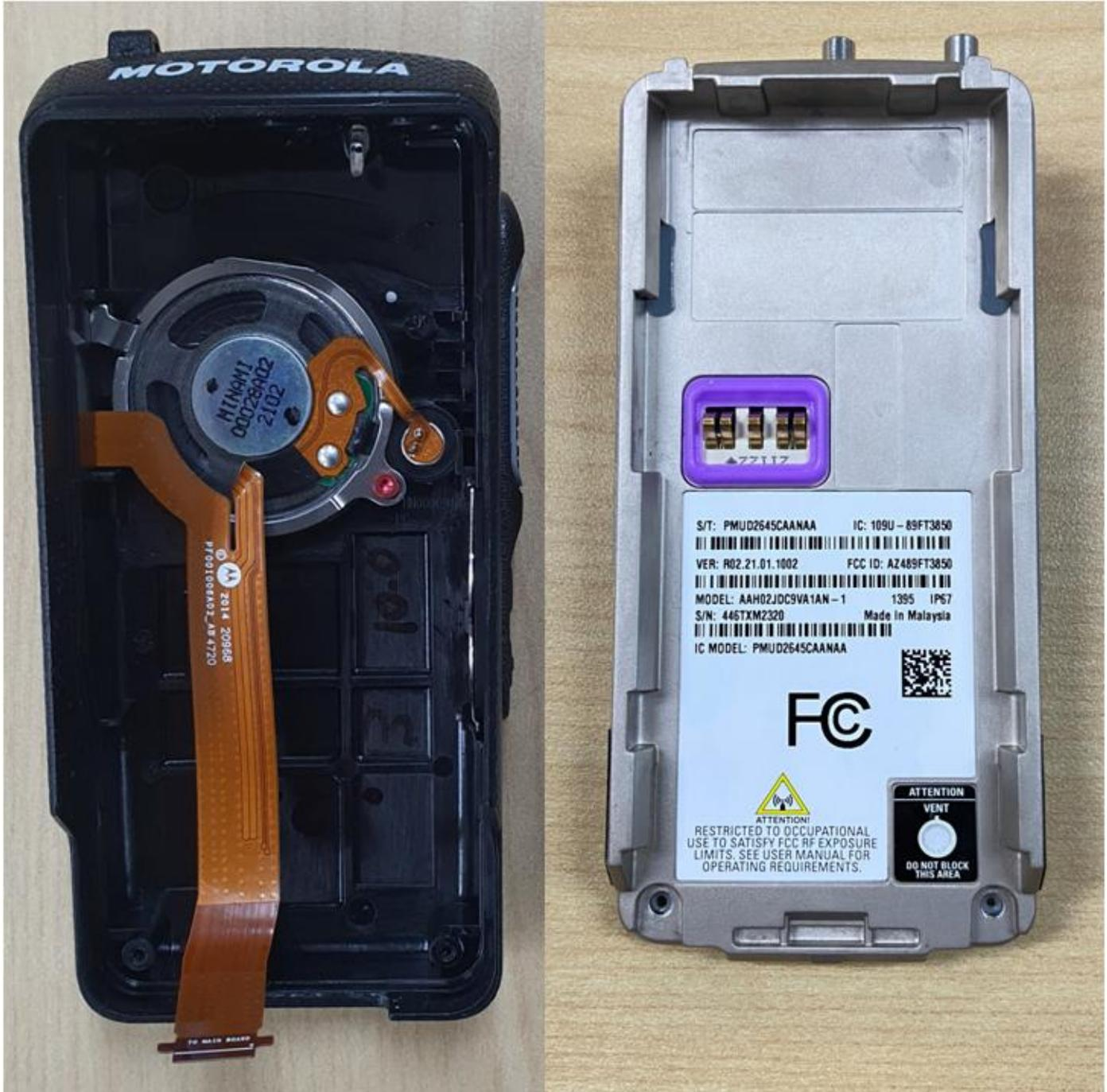
**Chassis and housing for Non Keypad model (Back Side) Non-TIA4950**
