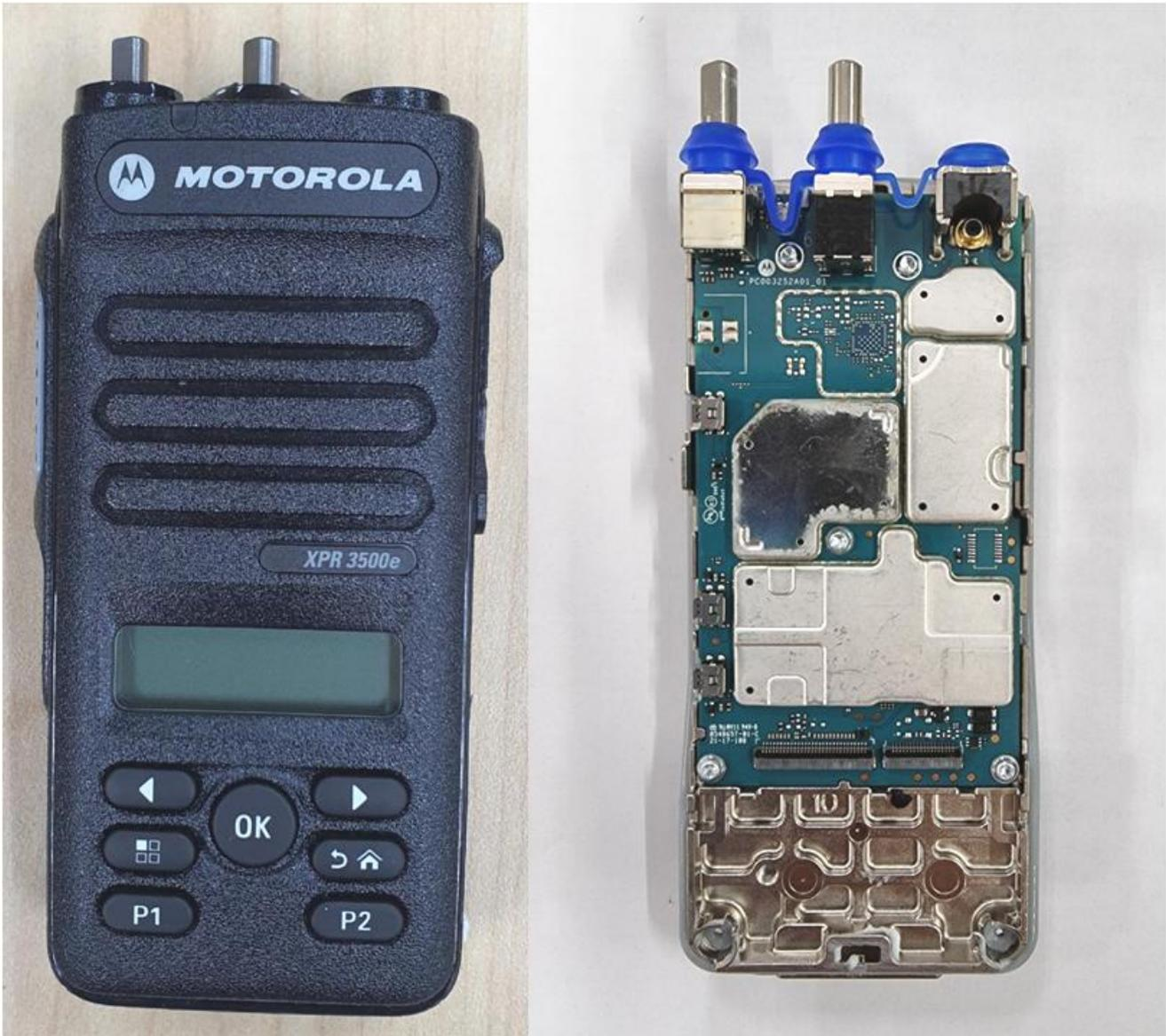
RF boards with chassis and housing for Display and Limited Keypad model (Front Side) TIA4950
