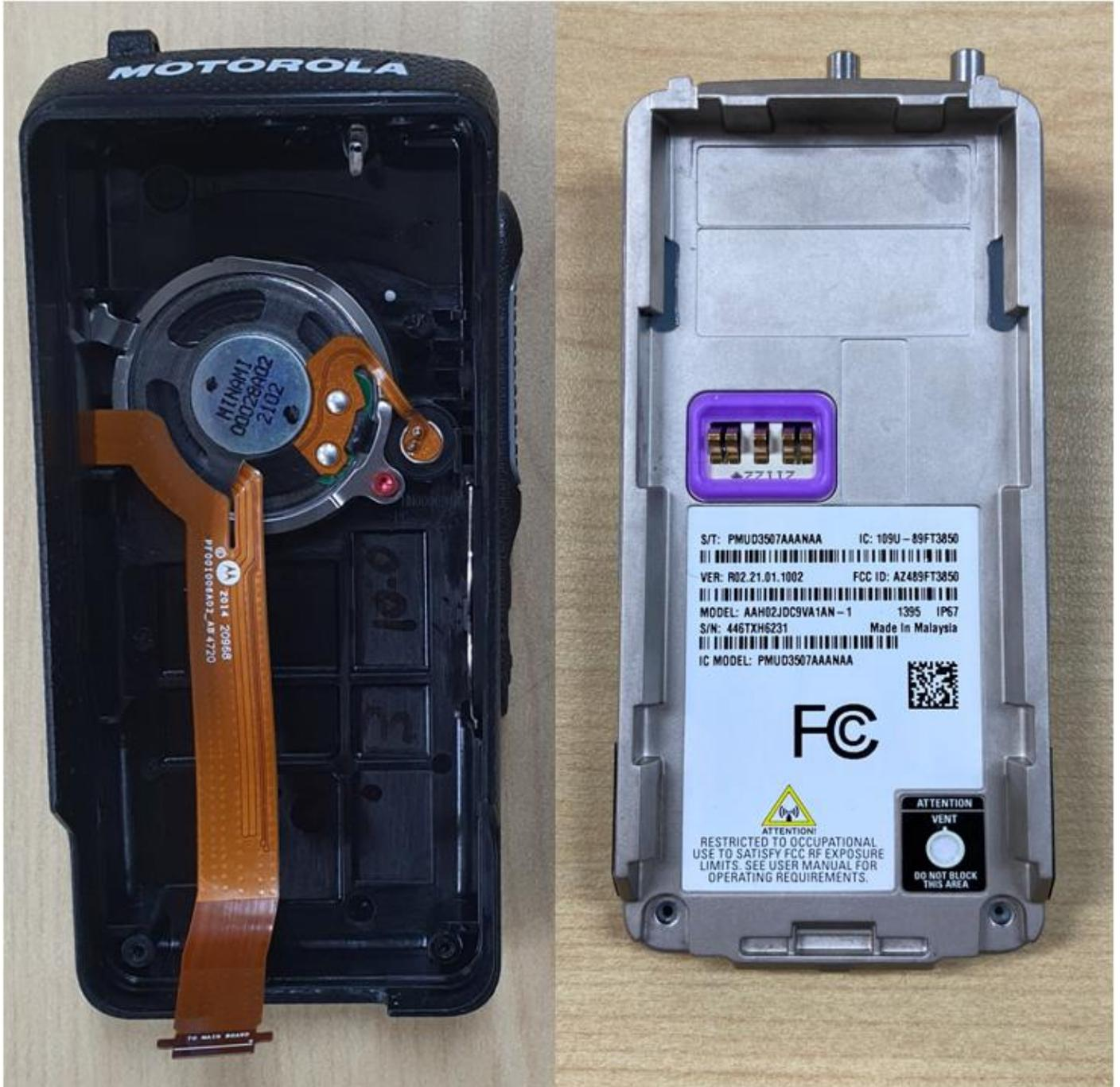
**Chassis and housing for Non Keypad model (Back Side) TIA4950**
