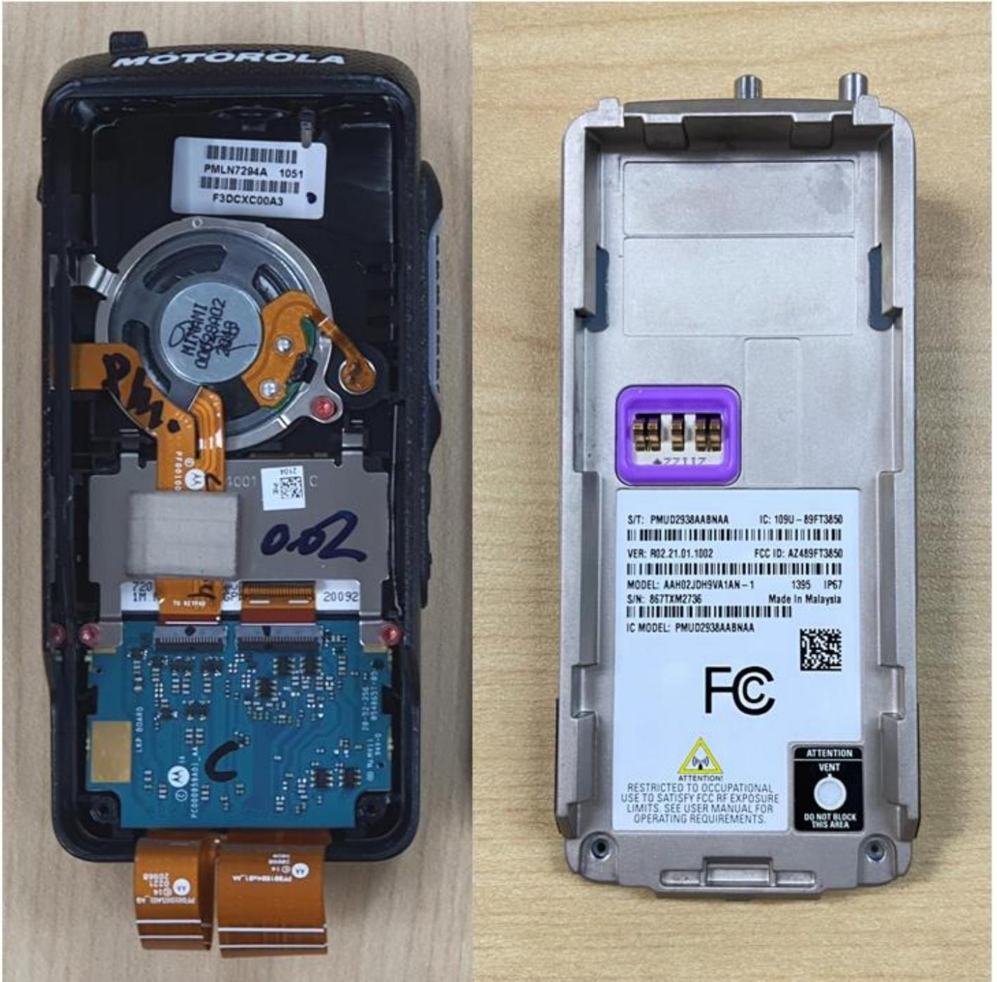
**Chassis and housing for Display and Limited Keypad model (Back Side) Non-TIA4950**
