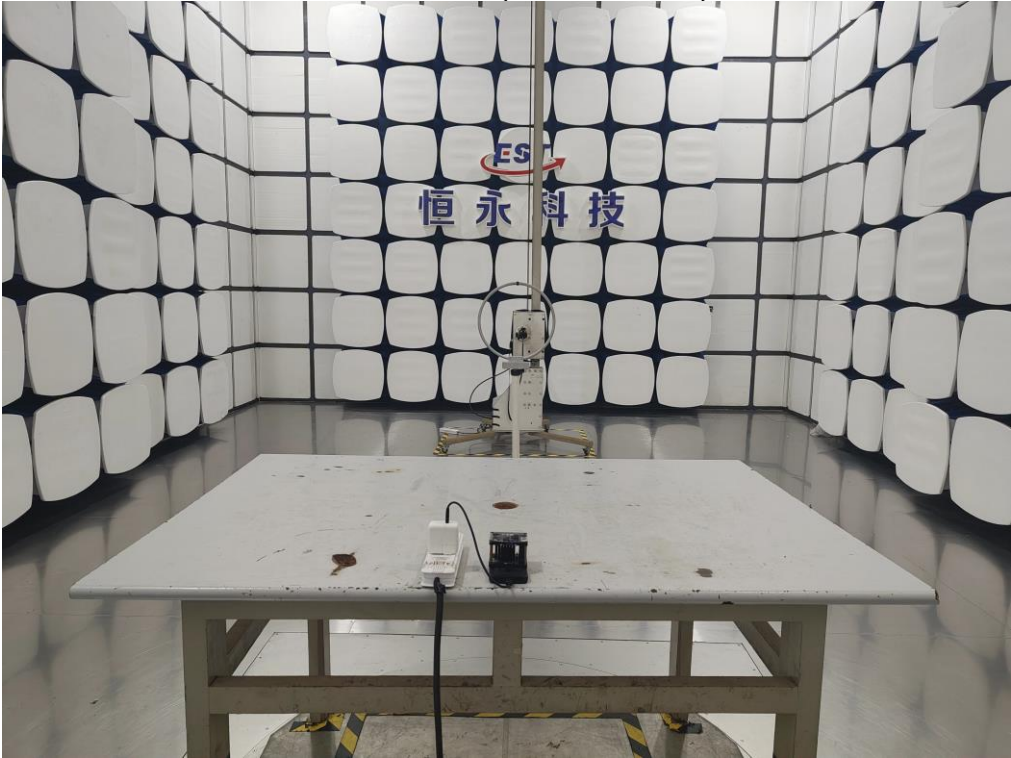
Radiated Test (Below 30MHz)
