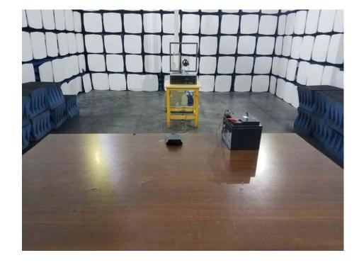
Spurious Radiation Test Setup (9kHz to 30MHz)
