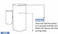
Blinking: The device enters pairing mode
