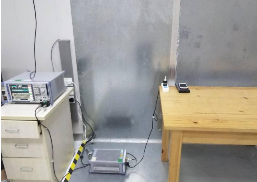
Radiated Spurious Emissions Test Frequency From 9kHz-30MHz
