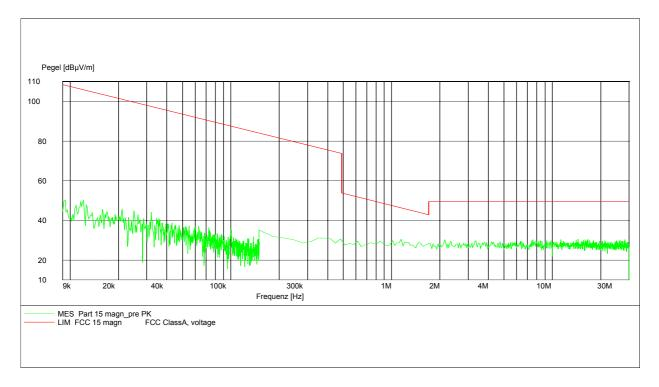
measured at a distance of 10m, recalculated to 30 or 300m with 40 dB per decade according to FCC rules.
