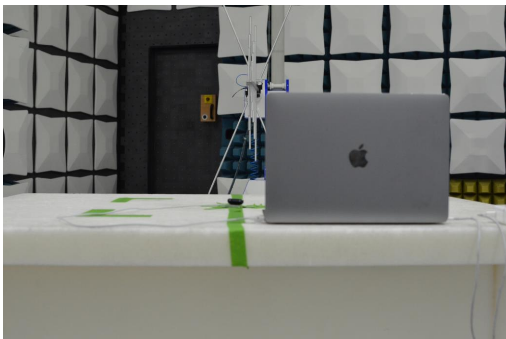
Figure 14: 30MHz-1GHz Test Setup (Rear View)
