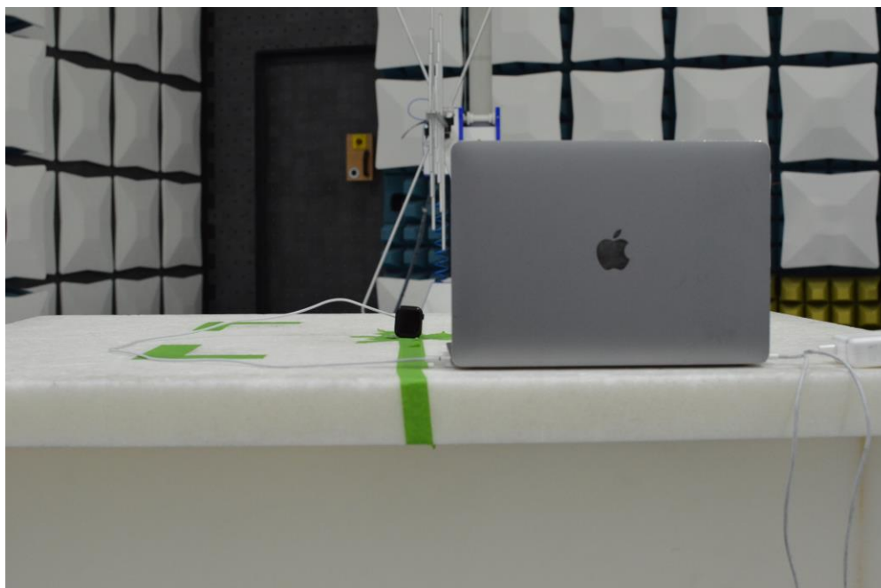
Figure 18: 30MHz-1GHz Test Setup (Rear View)
