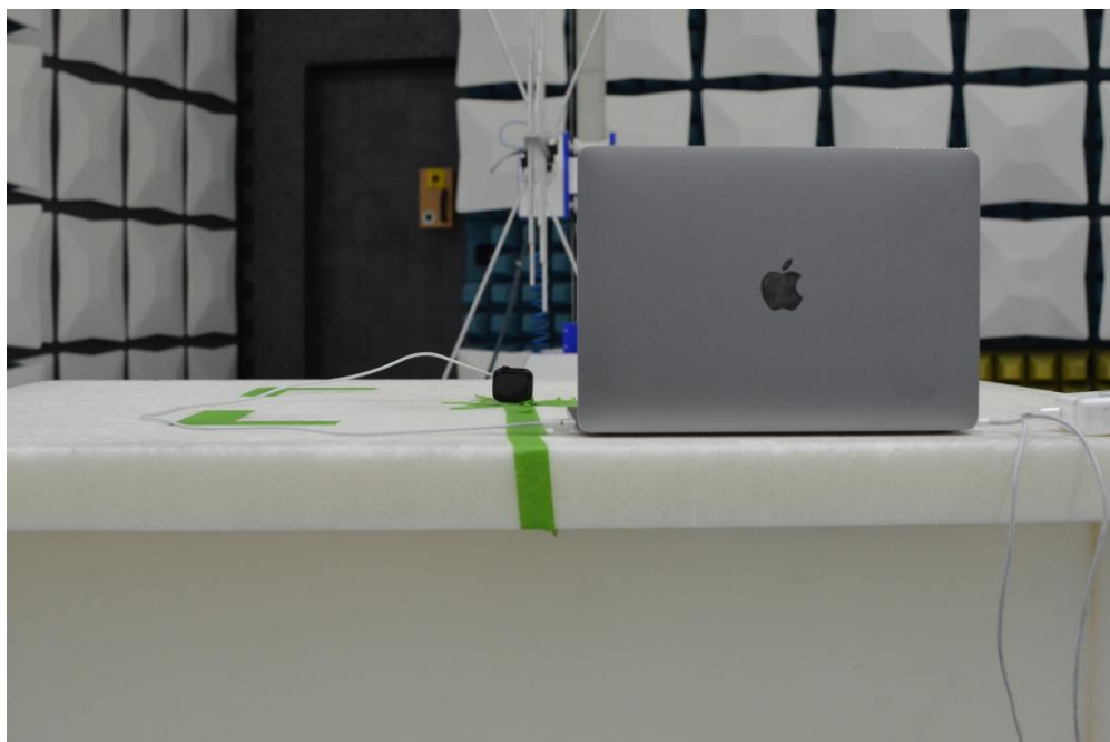
Figure 16: 30MHz-1GHz Test Setup (Rear View)
