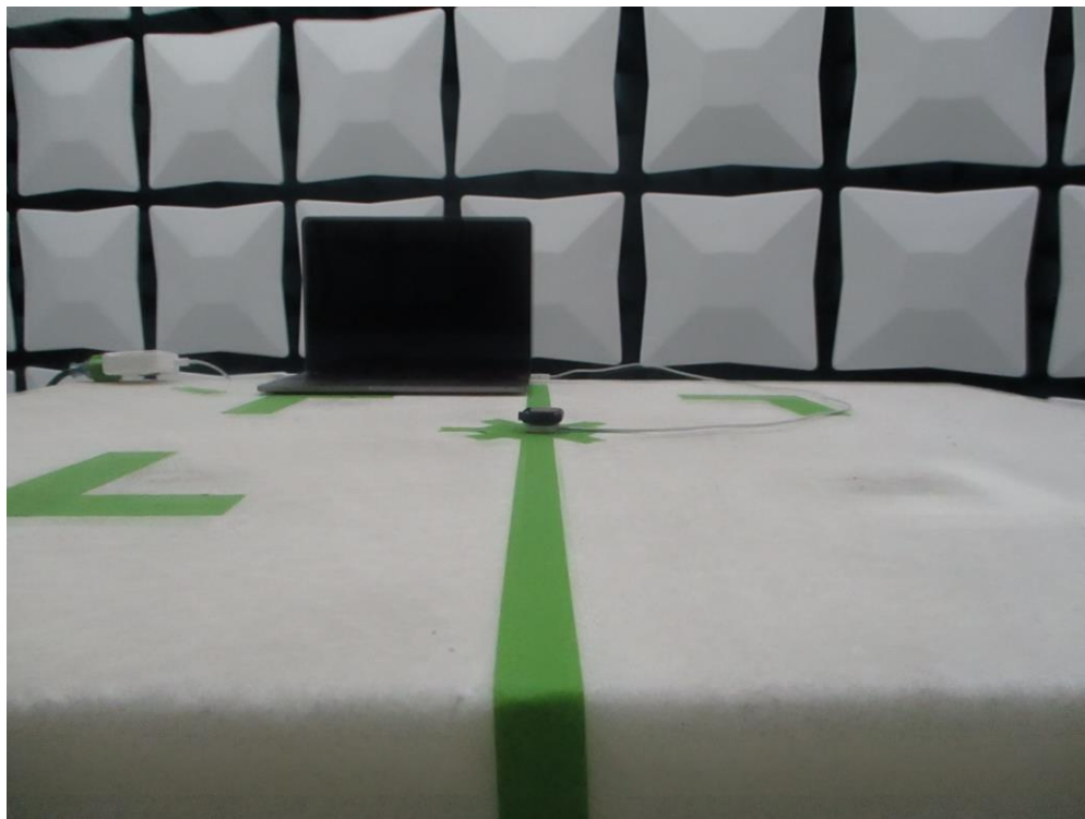
Figure 13: 30MHz-1GHz Test Setup (Front View)
