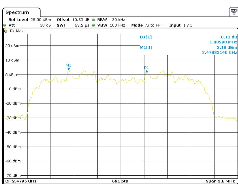
**EDR (8DPSK): Low Channel**
