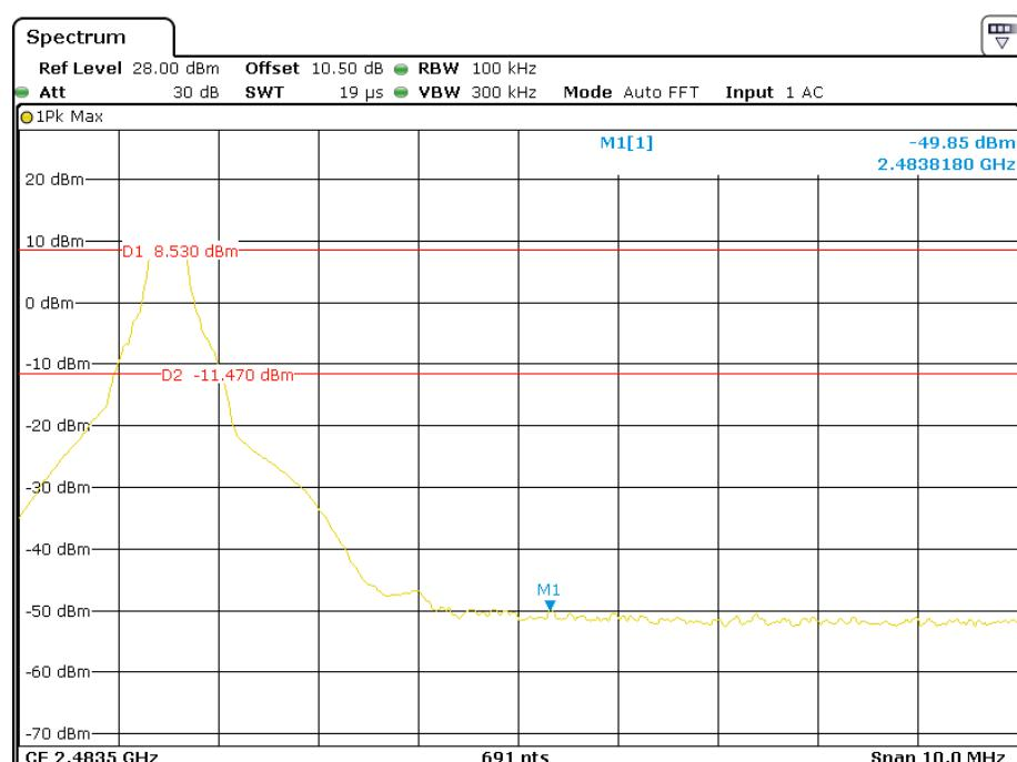
**EDR ( $\pi/4$ -DQPSK): Band Edge-Left Side Hopping**
