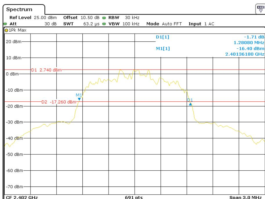
**EDR (8DPSK): Middle Channel**
