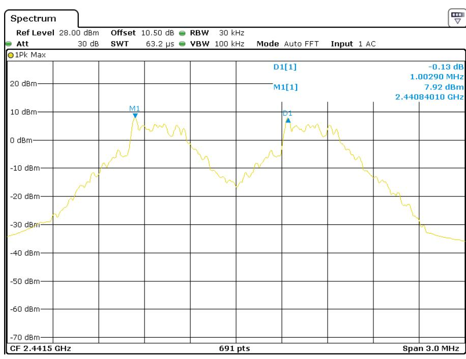
**BDR (GFSK): High Channel**
