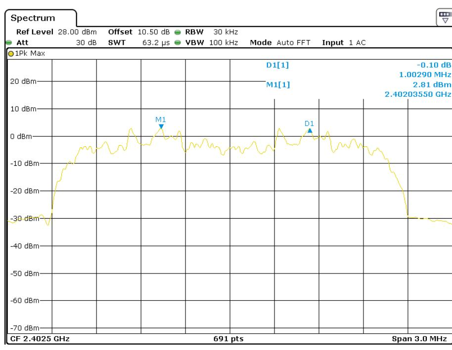
**EDR ( $\pi/4$ -DQPSK): Middle Channel**
