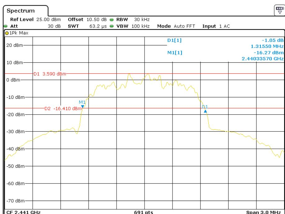
**EDR ( $\pi/4$ -DQPSK): High Channel**
