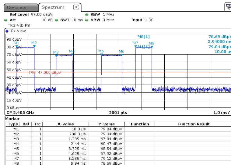
Note: The markers M3, M4, M5 and M6 are marker values according to the response of the companion device.
