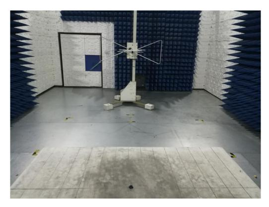
RADIATED EMISSION TEST SETUP ABOVE 1GHZ
