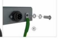
Connect and screw the ground wire to AU-PS.
