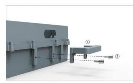
Fasten the handle to the side of MP-PS with 2×M6×14 screws.
