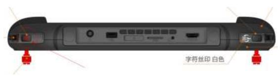
Power button of the android PAD, for power on and off, and close/on the LCD.
