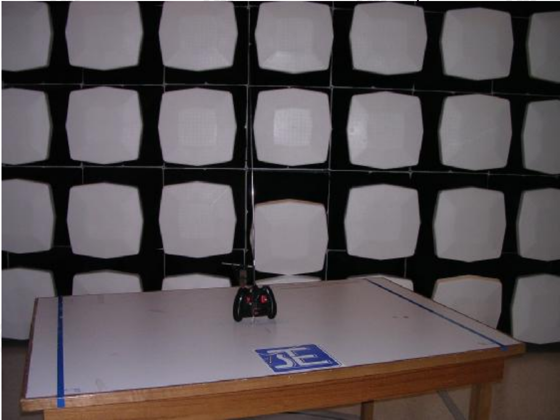
Measurement of Radiated Emission Test Set Up
