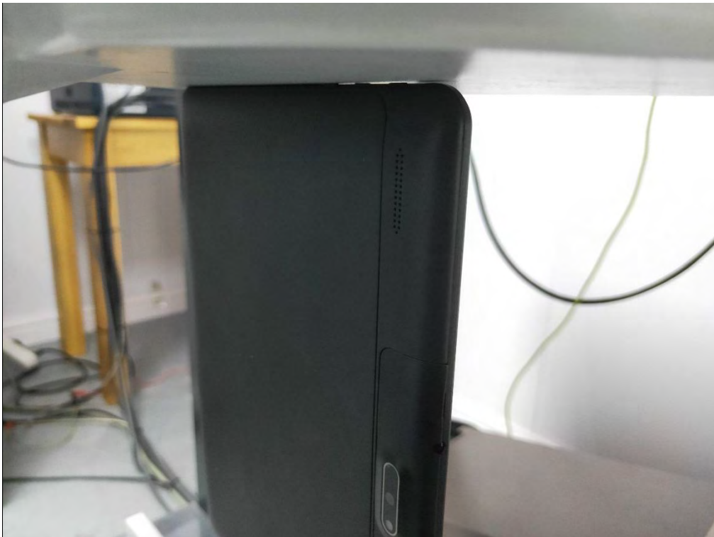
0mm body-worn Right Side Setup Photo (hotspot)
