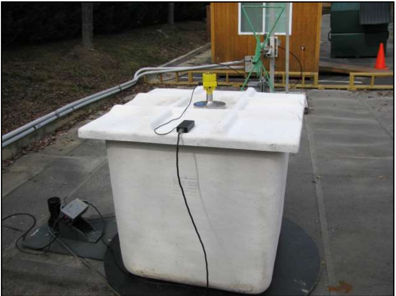
Photograph 16: Radiated Emissions – TC #3; Fiberglass Container
