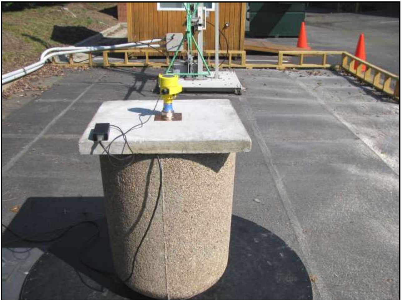
Photograph 8: Radiated Emissions – TC #1; Concrete Container
