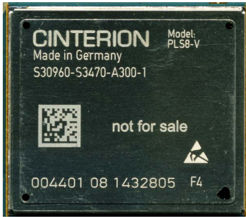
PLS8-V label location lasing on shielding
