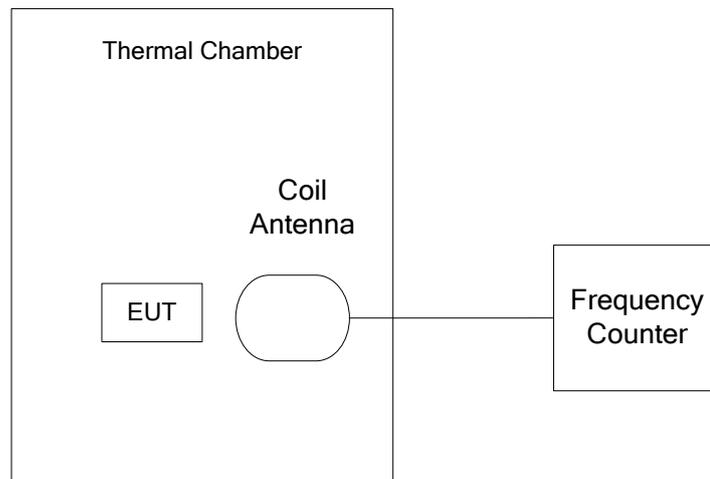
The transmitter output signal was picked up by coil antenna connected to the frequency counter. The center frequency was measured with 30Hz RBW and 1kHz span.
