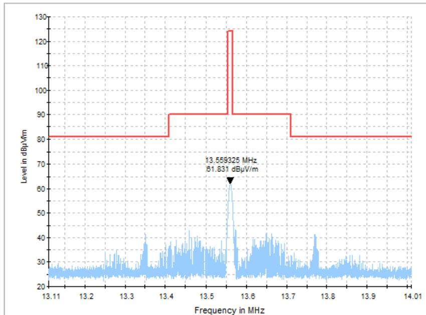
**Figure A-1 Electric Field Strength**
