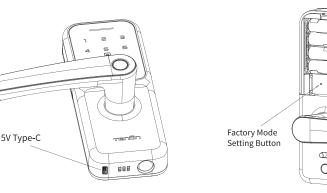
If the battery is dead, charge the lock with a 5V Type-C charging bank.
