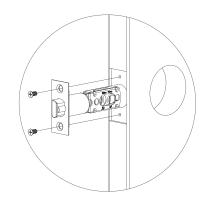
(4) Insert suitable threaded sleeves and square rods to the corresponding position of the front panel (As shown).
