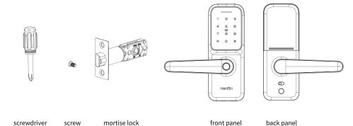
2 Modify the mortise lock backset based on the distance from the hole centerline to the door edge.
