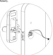
The back panel shall be connected with the wire of the front panel and the wire of the mortise lock(As shown).
