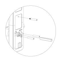
(5) Thread the front panel wire through the hole. The front panel square rod exits through the square rod hole of the mortise lock. (As shown).
