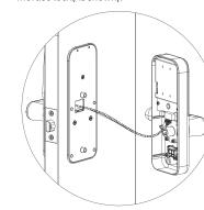
At last put into batteries and cover them. Move the anti-peep button right side to the unlocking position (as shown): Please check whether lifting handle can lock the door properly or pressing handle can open the door normally; Please check whether the unlocking ways of password, fingerprint, card and mechanical key can work properly.
