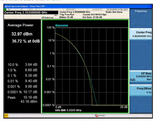
Port1 / LTE 5 MHz / 2 357.5 MHz / 64QAM
