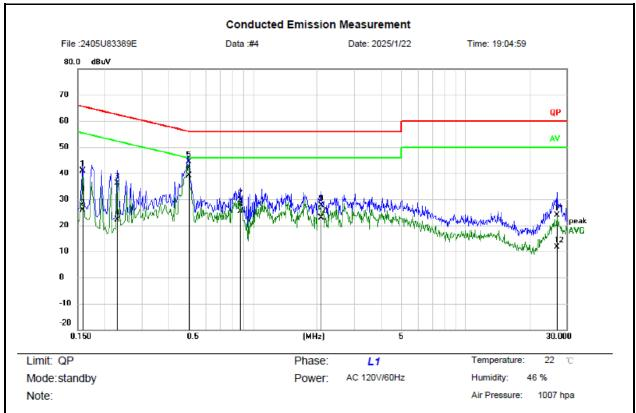
Receiver Setting: 9~150kHz: Pre-scan: RBW: 200Hz, DET: PK/AV; Final measure: RBW: 200Hz, DET: QP/AV 0.15~30MHz: Pre-scan: RBW: 9kHz, DET: PK/AV; Final measure: RBW: 9kHz, DET: QP/AV
