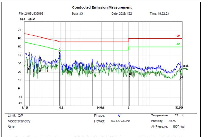
Receiver Setting: 9~150kHz: Pre-scan: RBW: 200Hz, DET: PK/AV; Final measure: RBW: 200Hz, DET: QP/AV 0.15~30MHz: Pre-scan: RBW: 9kHz, DET: PK/AV; Final measure: RBW: 9kHz, DET: QP/AV
