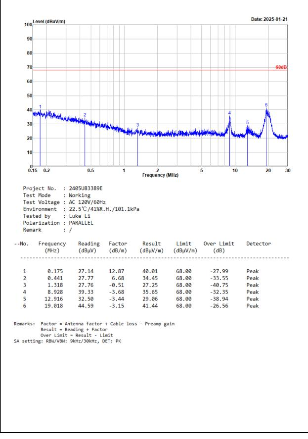
Note: According to FCC § 18.305, the field strength limit of the outside band emissions is: Limit=20lg(25)+20lg(300/3)=68dBuV/m
