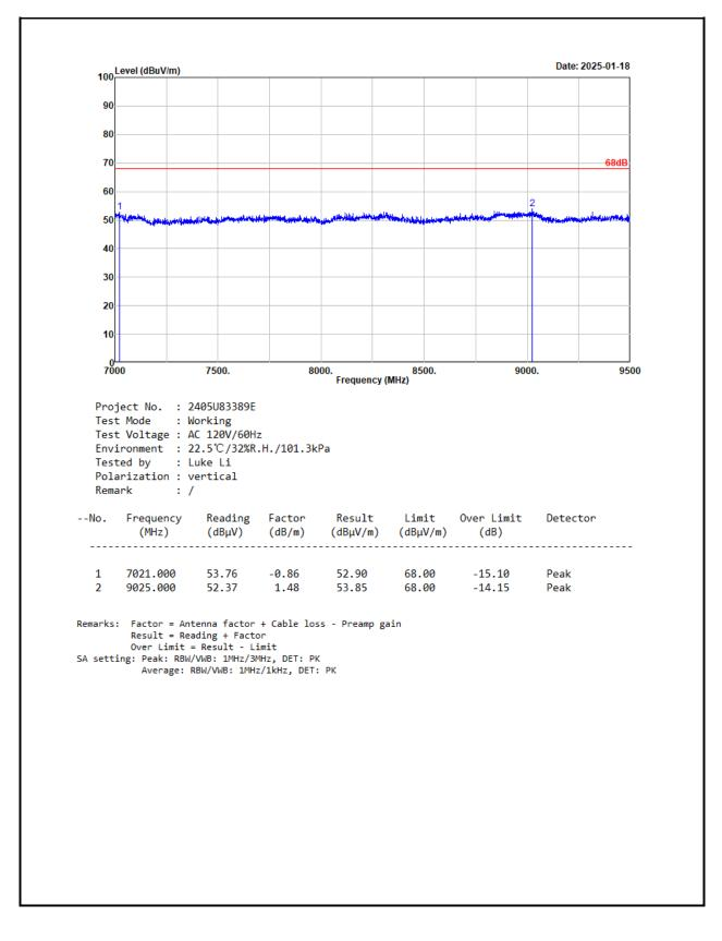
Note: According to FCC § 18.305, the field strength limit of the outside band emissions is: Limit=20lg(25)+20lg(300/3)=68dBuV/m
