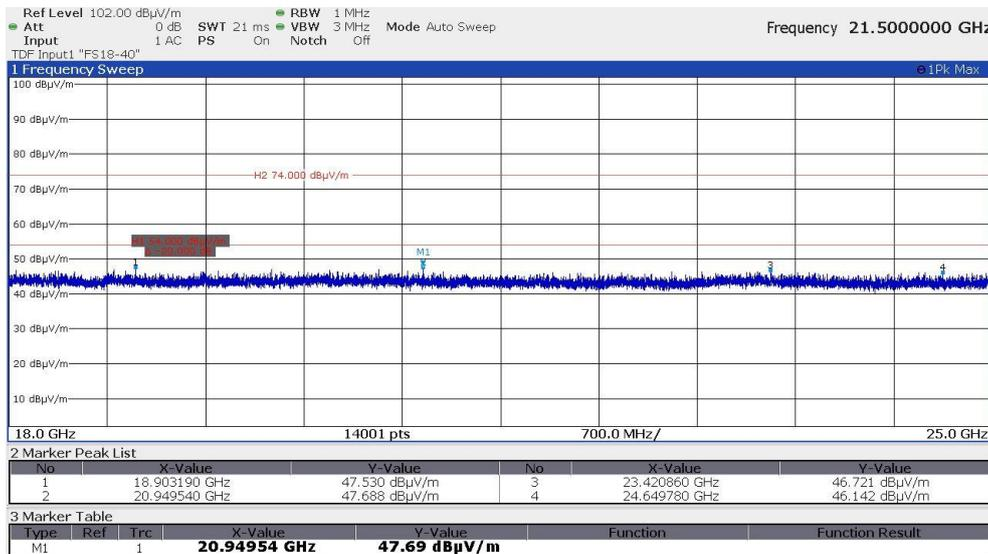
2) Measurements of emissions according to spurious emissions limit specified in section 15.247(d) / RSS-247 5.5:
