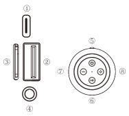
1.DC 5V slot: Use the standard Type C charging cable for power charging.
