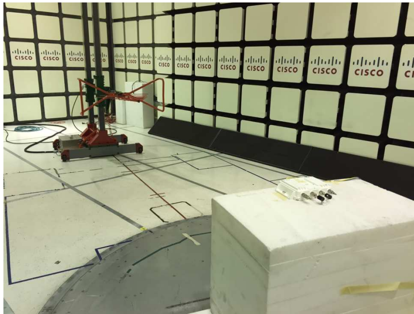
Title: Radiated Spurious Emissions Test Configuration 30M - 1000MHz
