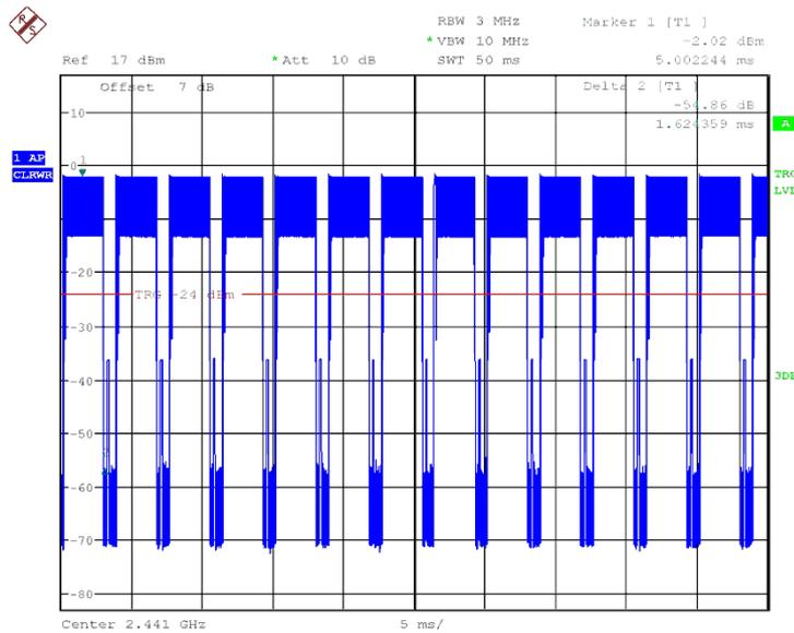
Fig.75 Number of Transmissions Measurement: Ch39, Packet 3-DH5
