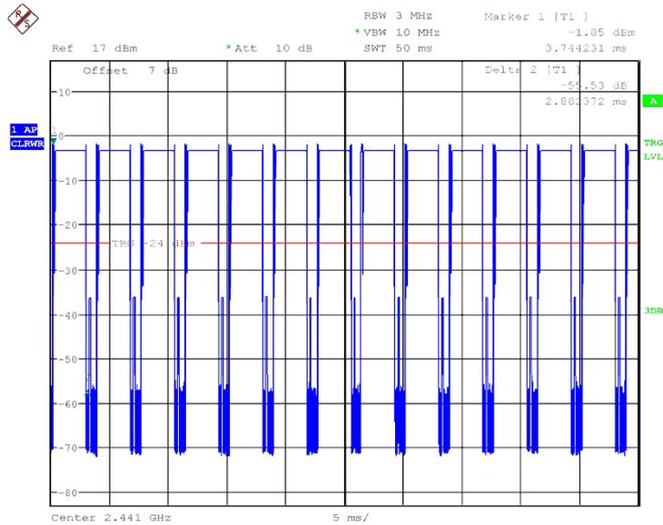
Fig.69 Number of Transmissions Measurement: Ch39, Packet 2-DH5
