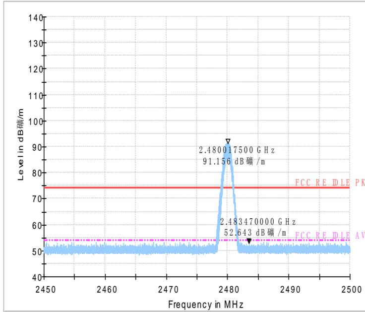
Fig.44 Radiated emission (Power): GFSK, high channel
