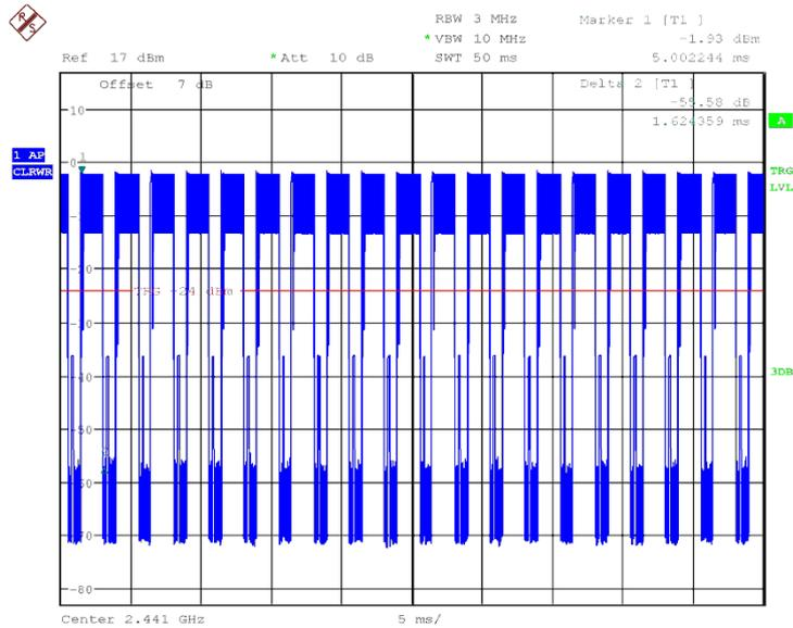
Fig.73 Number of Transmissions Measurement: Ch39, Packet 3-DH3
