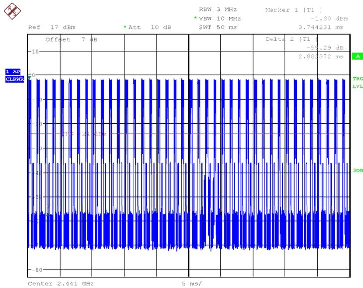
Fig.71 Number of Transmissions Measurement: Ch39, Packet 3-DH1
