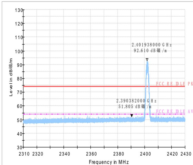
Fig.49 Radiated emission (Power):  $\pi/4$  DQPSK, low channel
