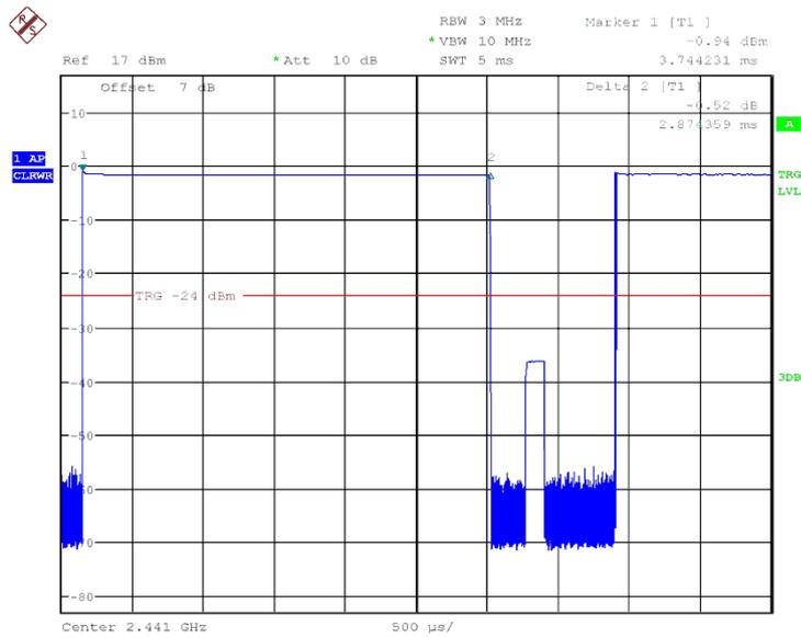
Fig.63 Number of Transmissions Measurement: Ch39, Packet DH5
