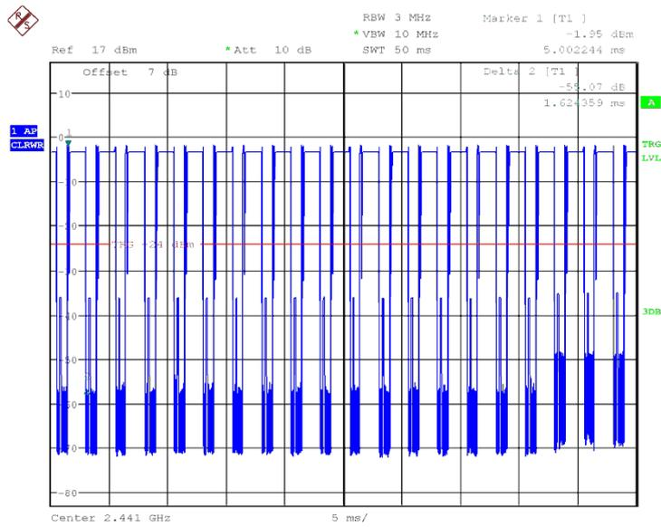
Fig.67 Number of Transmissions Measurement: Ch39, Packet 2-DH3
