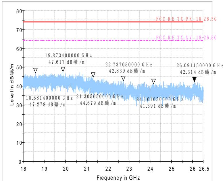
Fig.57 Radiated emission: 8DPSK, 18 GHz - 26 GHz
