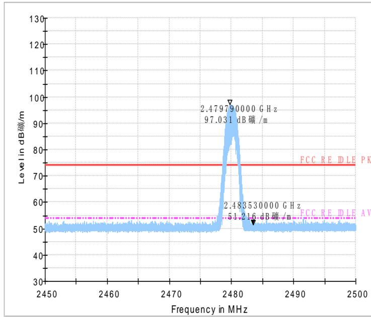
Fig.50 Radiated emission (Power):  $\pi/4$  DQPSK, high channel
