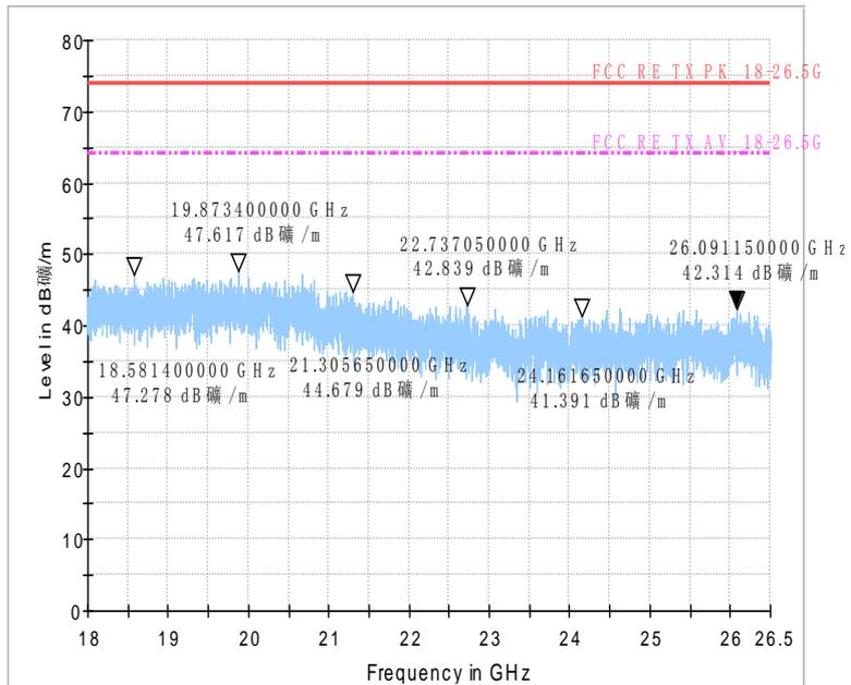
Fig.45 Radiated emission: GFSK, 18 GHz - 26 GHz
