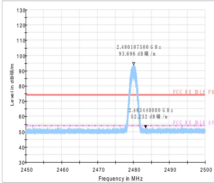
Fig.56 Radiated emission (Power): 8DPSK, high channel
