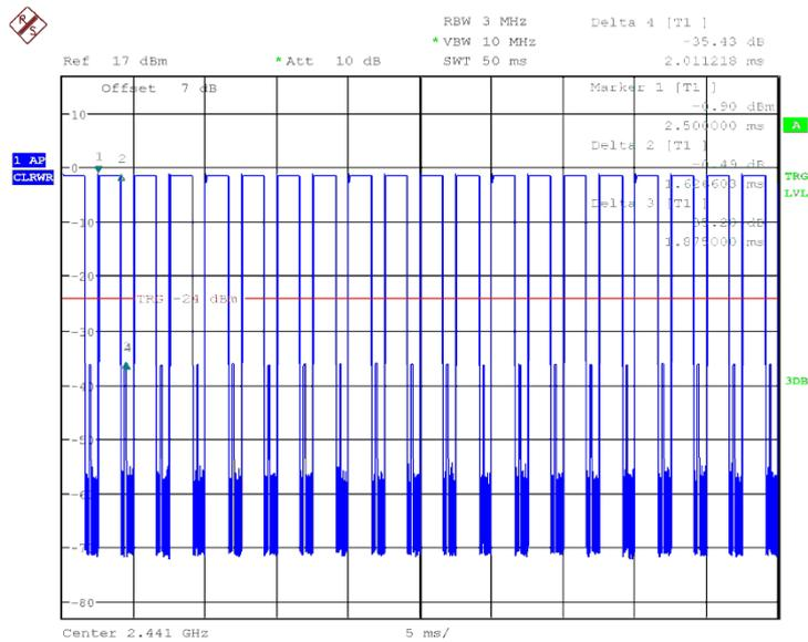
Fig.61 Number of Transmissions Measurement: Ch39, Packet DH3
