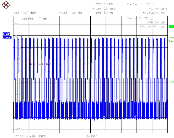
Fig.65 Number of Transmissions Measurement: Ch39, Packet 2-DH1
